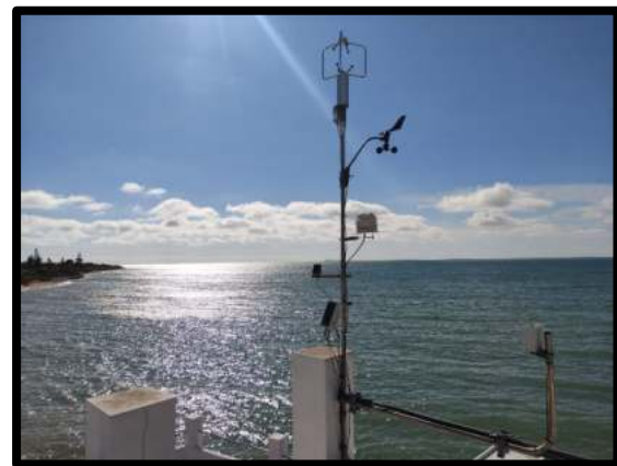
Fig. 2. Example of coastal observations that will be included in the new OceanUCA platform. In this case, the picture shows a remote automatic weather station installed in Chipiona, providing real-time data on wind speed, wind direction, temperature, humidity, pressure, and downward short-wave radiation data. Besides, this station has a 3D sonic anemometer at its top to calculate turbulence and surface heat flux data directly from high-frequency measurements (10 Hz) through the Eddy-covariance technique. These types of observations will be also included in the system.
