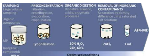
Fig. 1 Example of a sample preparation strategy for the extraction of microplastics from the seawater matrix (WP2).
