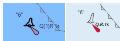
Figure 3. S-52 Buoy with red light flare (left) compared to an SVG of the same symbol in CCB (right). Lua script is used to replace the symbol for the object.
