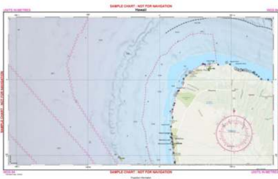
Figure 6. Custom product exported PDF with MCS, raster bathymetry, vector tile topography and hand-placed compass rose.
