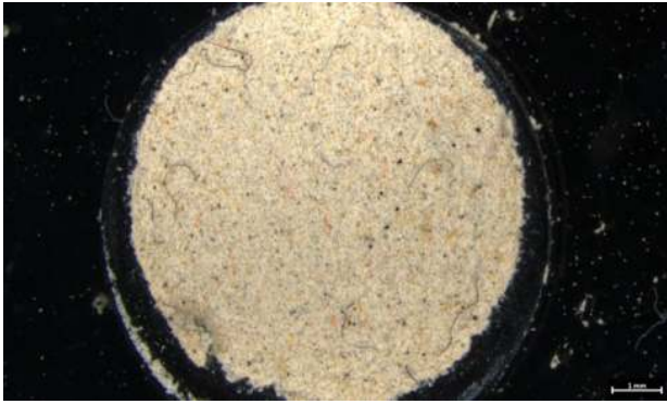
Fig. 4 Example of silicon membrane with a layer of SPM.
