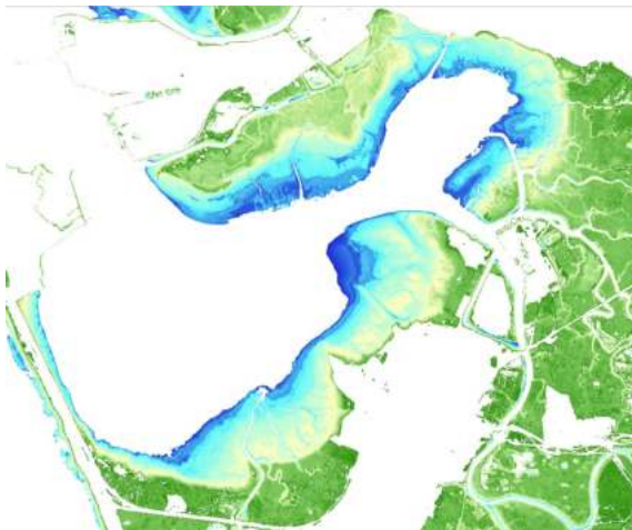
Fig. 3. Intertidal relief model obtained for the inner Cadiz Bay.
